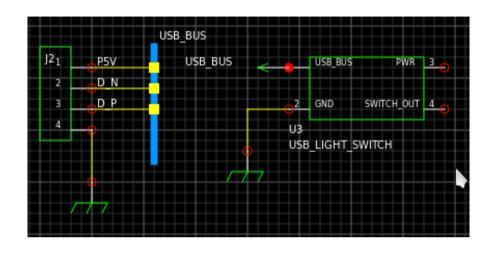
The pin's Connect to Bus popup option adds a net stub to the selected bus
